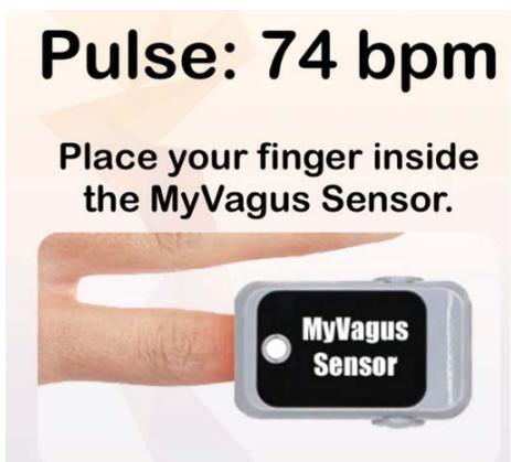
Figure 3 (a): MyVagus Sensor is a modified pulse oximeter used to capture PPG signal.
